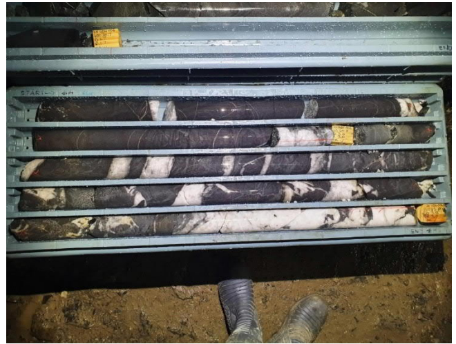
Figure 3: Eaglehawk reef showing typical mineralised quartz/sulphide lodes, UH-UDH-006: 59.73m to 61.5m for 1.77m @ 29.6 g/t gold
