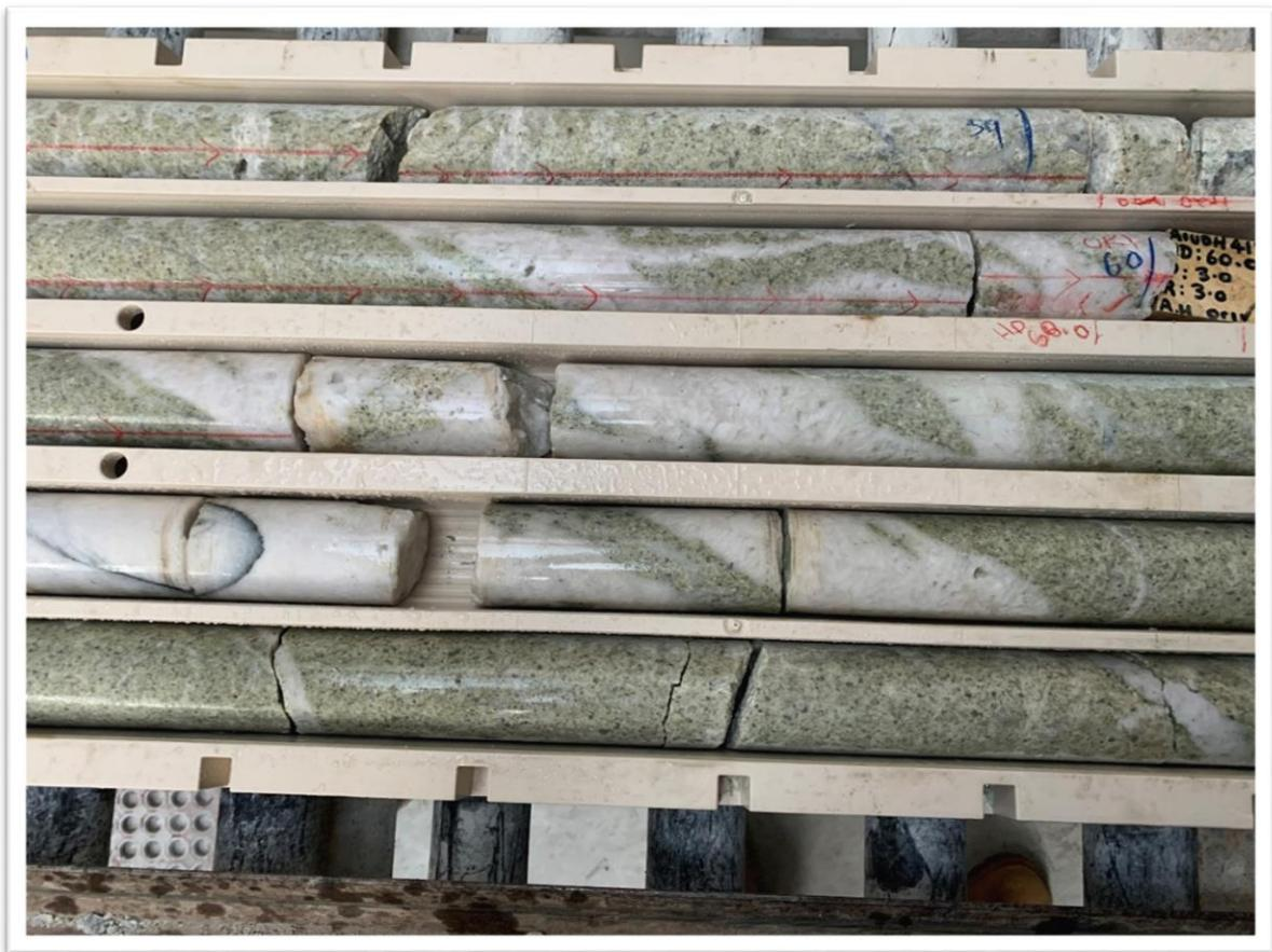
**Figure 1: Drill core from hole #417 showing intense alteration and bleaching of the diorite host and abundant quartz veining (~58.5 – 62.5m).**
