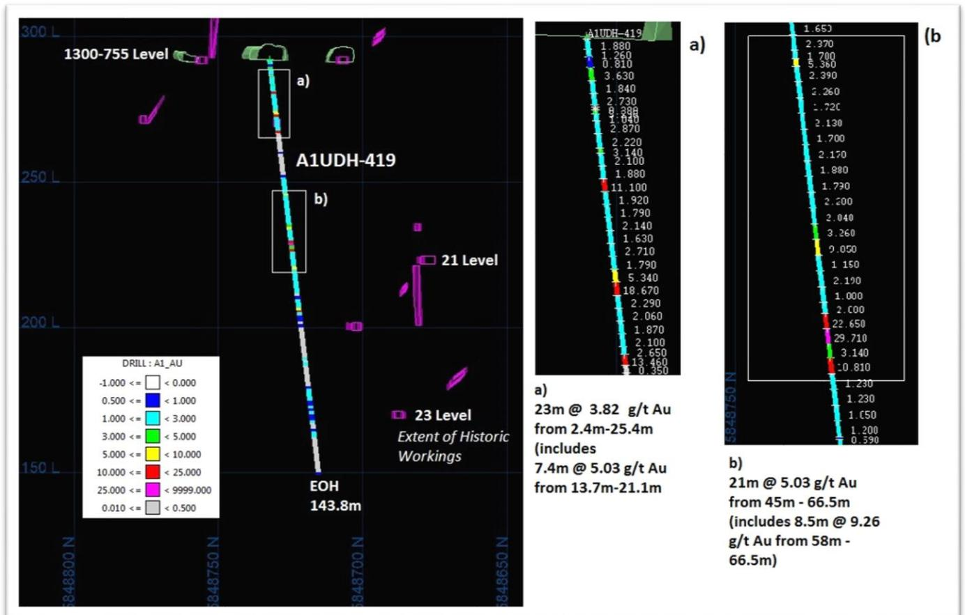
Figure 7: Trace and assays of drill hole A1UDH-419.
