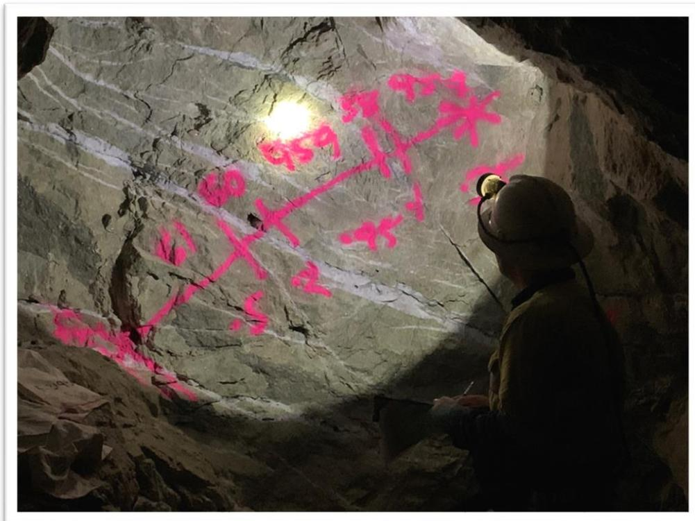
**Figure 3: Ore block marked for mining.**
