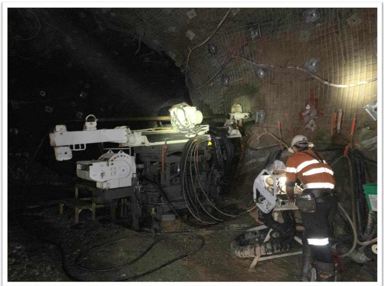
Figure 6: Underground diamond drilling at the A1 Mine.
