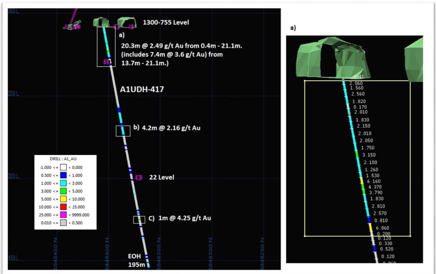
**Figure 8: Trace and assays of drill hole A1UDH-417.**
