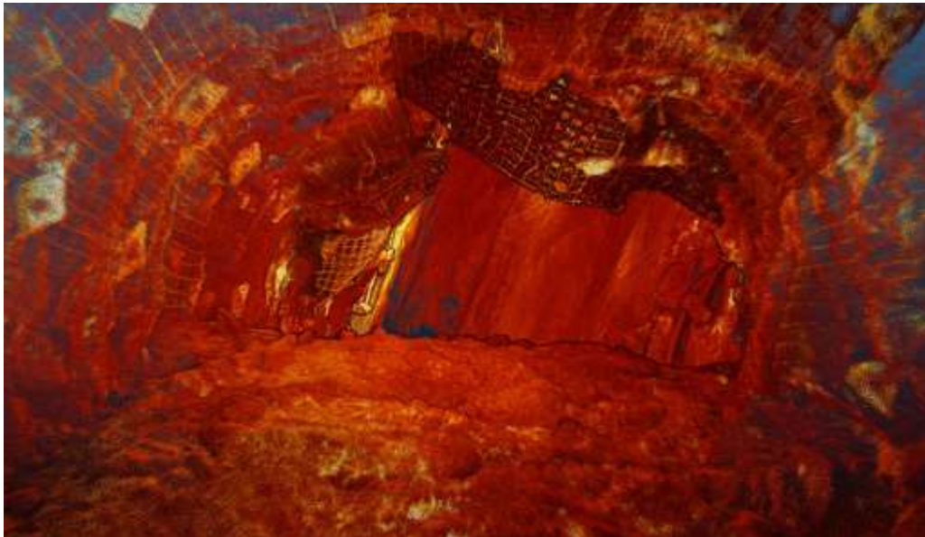
Figure 2: Example image of a drive being surveyed showing laser survey lines (not from Maldon)
