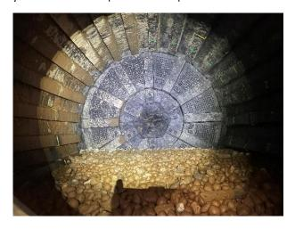
Figure 3. New Mill liners installed
