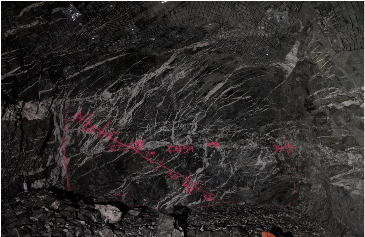
Figure 2: Showing a 5.1m high face from the 1237 Level SP22 Heading - interpreted to represent the Neesham Lode
