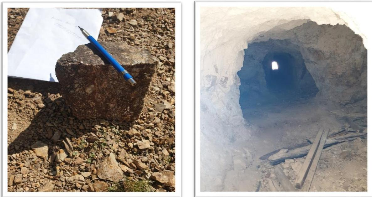
**Figure 5: Left; Rhyolite breccia taken from the Specimen Hill Mine. Right; View from inside the Specimen Hill Mine; the walls are sulphide rich brecciated rhyolite and gold bearing quartz veins.**
