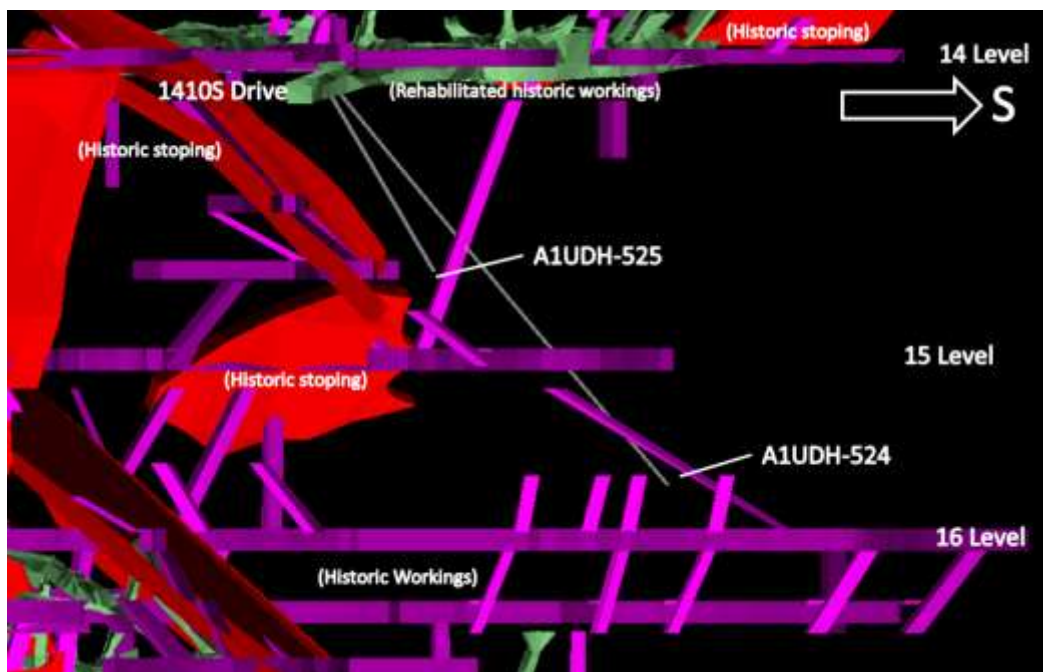
Figure 10: Long section looking East showing drilling traces, modern drives (green) and the interpreted historic workings (magenta) and stoping (red).
