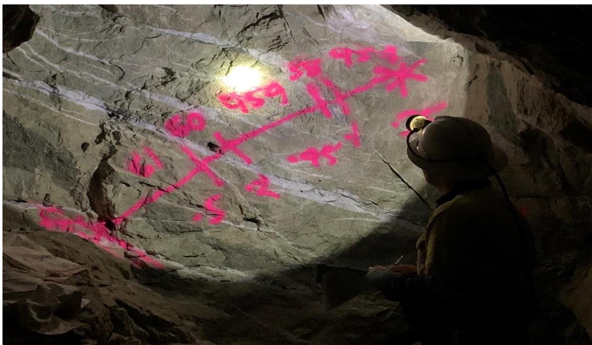
**Figure 1: Ore block marked for sampling.**
