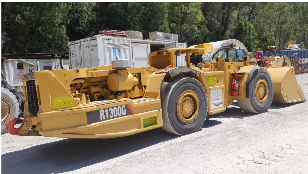
Figure 3: First of the expanded mining fleet (remote capable) has arrived on site to support future increased production- CAT 1300 LHD.
