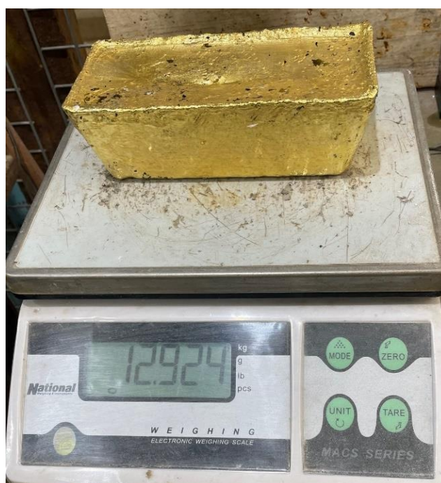
Figure 1: Record weekly pour showing gold dore (unrefined gold) before final processing and refining.
